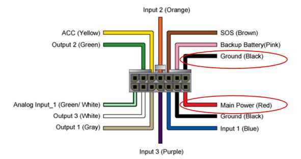
Connect the red wire from the cable to a power source of  $10\sim36$  V. Connect the black wire to ground.
