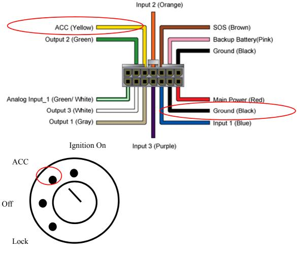
Connect the yellow wire from the cable to ACC/Ignition (12V) position of vehicle/asset. Connect the black wire to ground.
