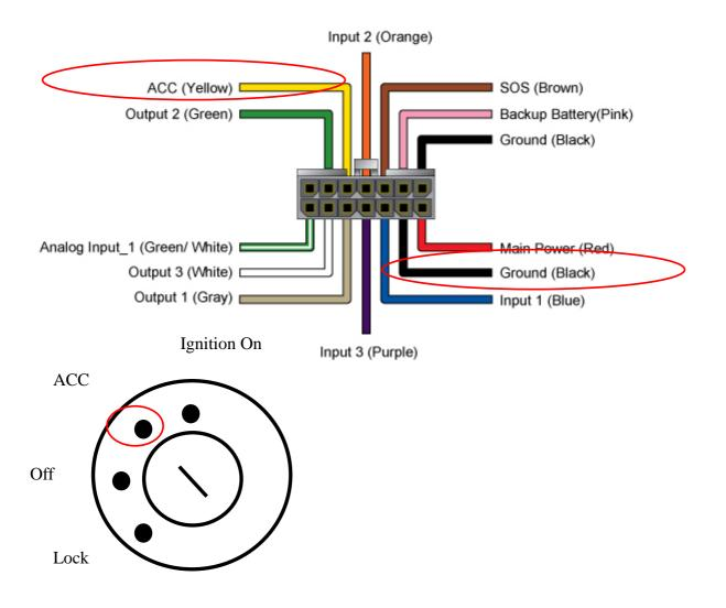
Connect the yellow wire from the cable to ACC/Ignition (12V) position of vehicle/asset. Connect the black wire to ground.
