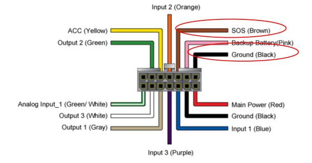
There is a line of the 14 pin IO cable for connecting push button for emergency help.
