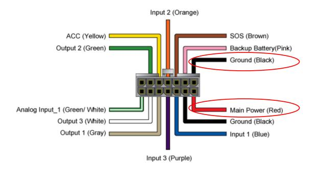
Connect the red wire from the cable to a power source of 10~36 V. Connect the black wire to ground.
