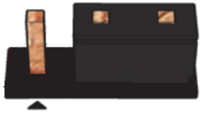
Pins 2&3: jumper position for 19V
