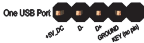
Figure 3 Front panel USB header pin-out
