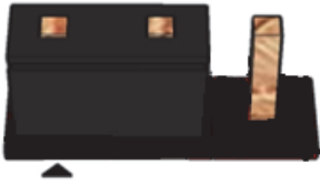
Pins 1&2: jumper position for 12V
